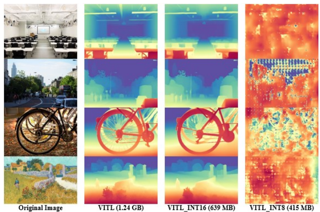
Figure 3. The dynamic INT16 model, with half the size, shows a great overall performance. The model capture global depth, but missing a few fine-details.
